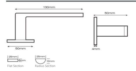
62001 Flat section 19mm lever handle on 50x4mm rose 62001D Radius section 19mm lever handle on 50x4mm rose
