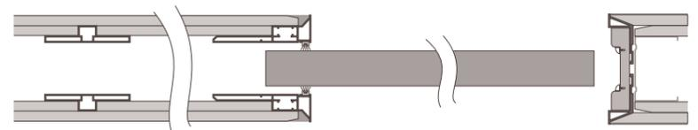
Double boarded wall - two 15mm plaster boards or one 18mm timber board and 12.5mm plaster board
