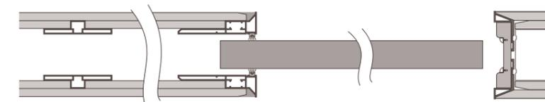
Double boarded wall - two 15mm plaster boards or one 18mm timber board and 12.5mm plaster board
