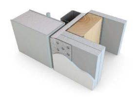
The Novista Riser system as standard has a frame with a perforated flange with an integral corner bead that sits on the face of the plasterboard or block wall, and this is then plastered or tape and jointed. The frame is manufactured from galvanised steel and this is supplied either factory painted or primed.
