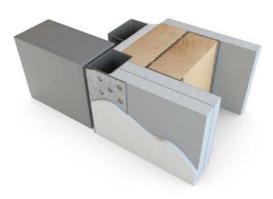
The Novista Riser Timber doorset has a frame with a perforated flange with an integral corner bead that sits on the face of the plasterboard or block wall, and this is then plastered or tape and jointed. The frame is manufactured from galvanised steel and this is supplied either factory painted or primed.
