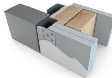
The Novista Riser Timber doorset has a frame with a perforated flange with an integral corner bead that sits on the face of the plasterboard or block wall, and this is then plastered or tape and jointed. The frame is manufactured from galvanised steel and this is supplied either factory painted or primed.
