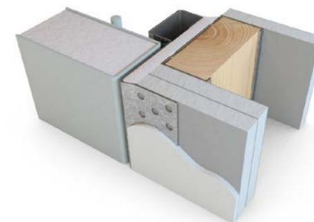
The Novista Riser system as standard has a frame with a perforated flange with an integral corner bead that sits on the face of the plasterboard or block wall, and this is then plastered or tape and jointed. The frame is manufactured from galvanised steel and this is supplied either factory painted or primed.
