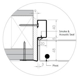
**Frame** Concealed/Picture frame design made from 1.2mm steel. 3 or 4 sided frame options
