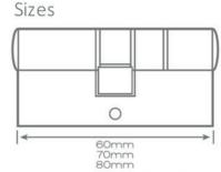
(Non-standard & offset cylinder lengths are also available in increments of 5mm)
