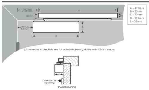
44007 adjustable power backcheck delayed action guide rail door closer - stainless steel
