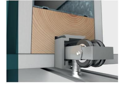
silent The aluminium track is mounted within a timber beam and this, together with the nylon wheels, ensures silent operation.
